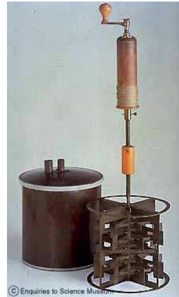
Joule's paddle wheel apparatus
